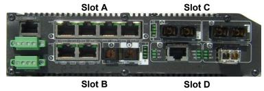
Step 4. Slot D: Choose one module *from the Step 2 list,* (OR choose from the following for Gigabit. (Gb is only available in slot D. No PoE in slot D).
