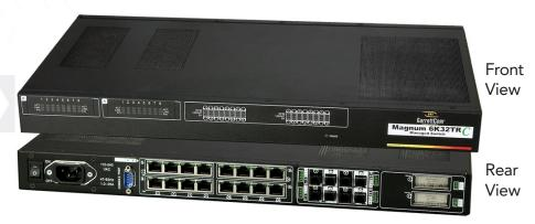
The Magnum™ 6K32TRC Switch provides rack-mount space efficiency in a free-convection-cooled unit (no fans) for heavy duty industrial applications where the presence of dust and dirt may inhibit normal cooling. New static thermal design techniques (patent pending) enable the 6K32TRC to deliver high reliability even at extended operating temperatures. Special rack-mount cooling techniques include
