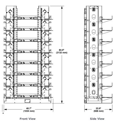
\* Add 3.25" (82.6 mm) when installing end guard.
